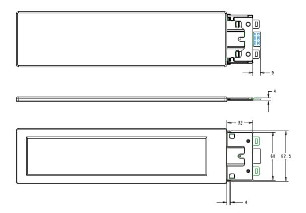
Figure 5: Keuka Module complete with Lampholder
