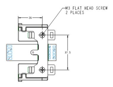
Figure 7: Contact pads of the Keuka Module Lampholder
