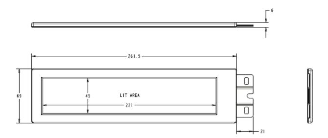
Figure 4: Keuka Module – front and side view
