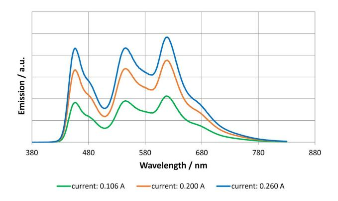
Figure 11: typical emission spectra of the Brite FL300 L ww at different driving currents (I = 0.135 A, 0.240 A, 0.368 A)
