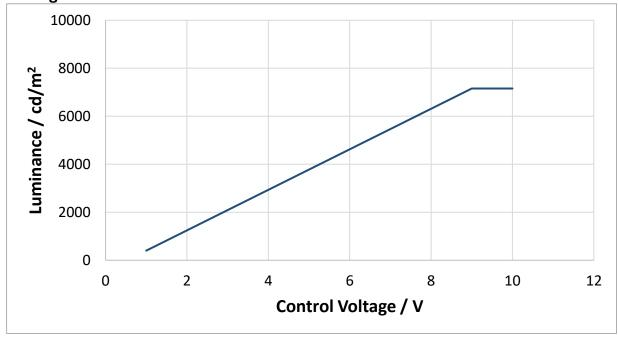
Figure 12: Luminance versus control voltage at room temperature
