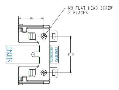
Figure 3: Lampholder complete
