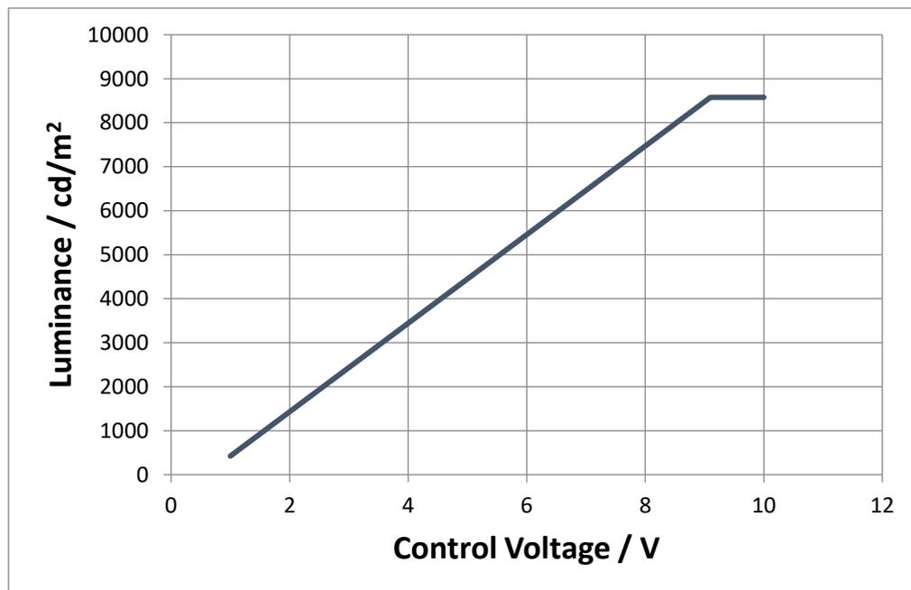
Figure 12: Luminance versus control voltage at room temperature
