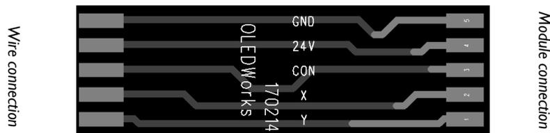
Figure 7: Contact pads of the Keuka Module Lampholder
