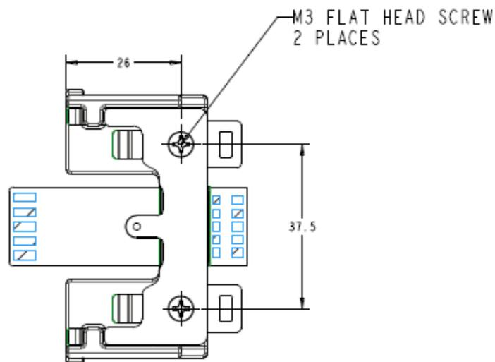
Figure 7: Contact pads of the Keuka Module Lampholder
