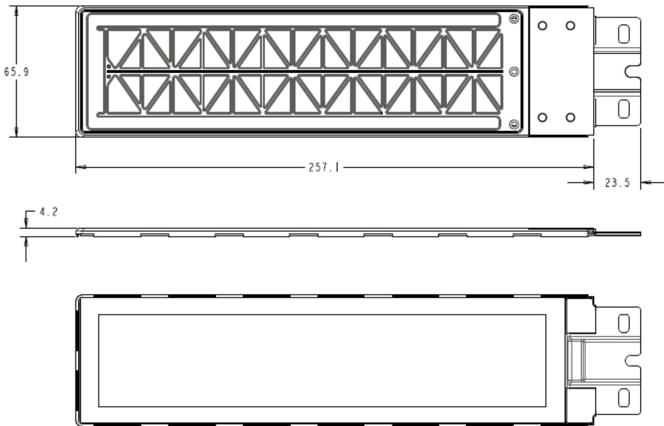
Figure 2: Keuka Module Subassembly (front, side and back view)
