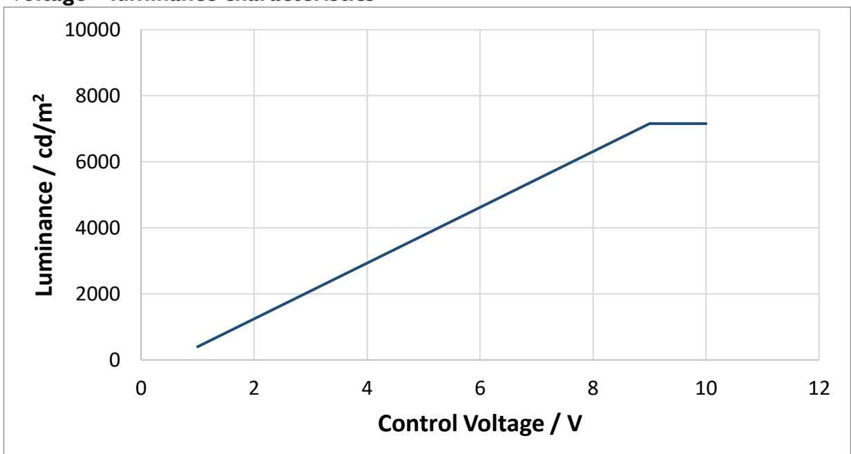
Figure 12: Luminance versus control voltage at room temperature
