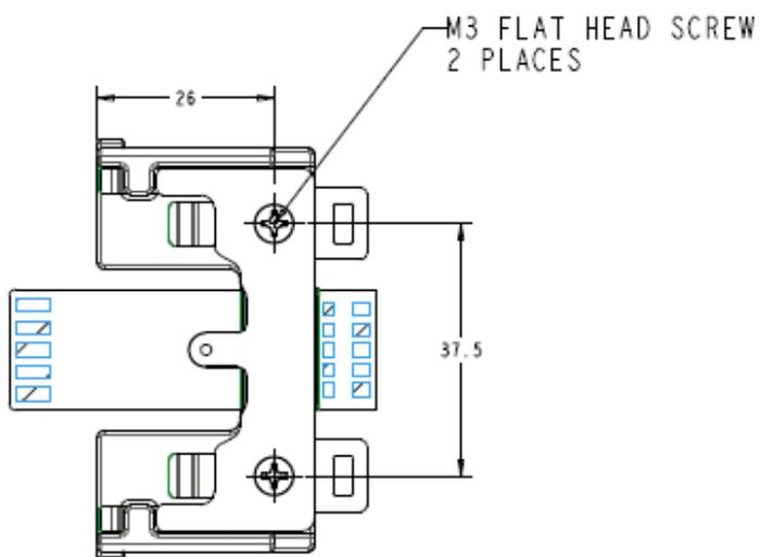
Figure 3: Lampholder complete
